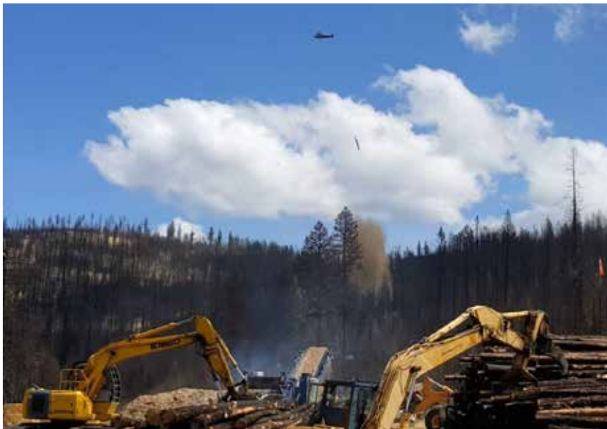
Figure 4. Wood shred mulch grinding and spreading via helicopter, Stickpin Fire, WA. Photo credit: Jason Jimenez, Colville NF.
